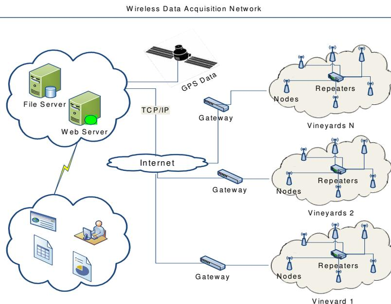
**Fig 1:** A schematic diagram of WSN layout for modeling the influence of climate change in weather, atmospheric and environmental conditions and on grapevine varieties and wine quality in different styles. The WSN transmits real time data collected through remote, wireless telemetry devices via repeaters, gateways and the Internet to a central sever for display and comparative analysis on the variability in climate change across the world's major wine regions and grapevine varieties.
