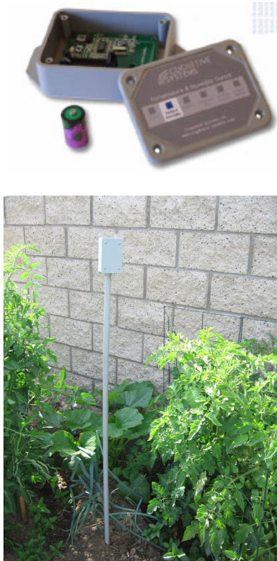
Fig. 2: WSN unit with microprocessor, transmitter, battery and built-in sensors for monitoring atmospheric temperature and humidity and wired sensors for wind speed/ direction and
